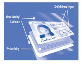
An example of the Integrated Circuit construction, where DEFENDER™ shielding can protect the card's sensitive information.
