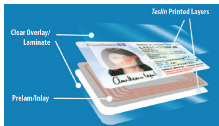
An example of Integrated Circuit construction, where DEFENDER™ shielding can protect the card's information.
