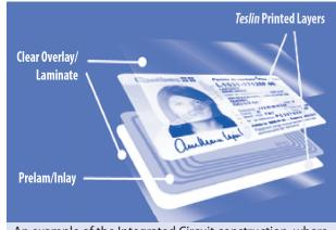
An example of the Integrated Circuit construction, where DEFENDER™ shielding can protect the card's sensitive information.
