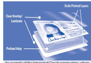
An example of the Integrated Circuit construction, where DEFENDER™ shielding can protect the card's sensitive information.
